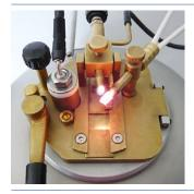
The instrument is equipped with two ignition systems. An electric pilot that ignites the test flame 30 seconds before the test.
