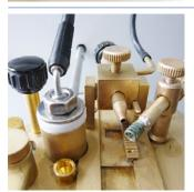
The ionisation components are the essential flash point detection system that grants excellent results and high repeatability. The quantity of sample (2 ml / 4 ml) is injected into the cup throught the filling orifice.
