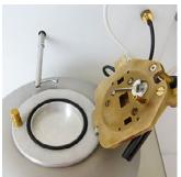
The test cup is completely made of aluminium and is equipped with a high temperatures resistant o-ring, allowing an uniform sealing of the closing cover.
