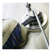
With the pliers the nut of the crucible cover is accurate and easily fixed.
