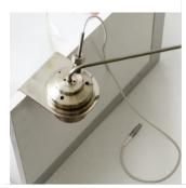
Crucible holder made in stainless steel keeps the cup assembly ready to use.
